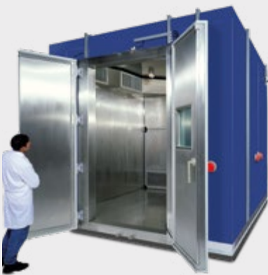
Walk-in chamber equipped with indirect cooling system to test specimen (base station) with high heat dissipation
