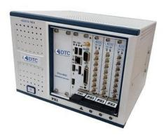
VESSTA MIMO Vibration controller is based on PXIe Bus and DSP board Structure, by the combination of different data acquisition card and output interface card, it can realize large-scale-channel distributed data acquisition, centralized processing, one-way transmission speed is up to 250 MB/s, it can ensure the multichannel parallel acquisition and real time closed-loop control.
